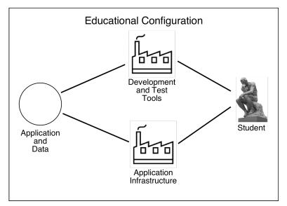
In the best instances of the educational configuration the development tools and the application infrastructure are tightly integrated, and moving between them is easy and fluid. Tools designed specifically for this kind of integration are Scratch<sup>5</sup> and Smalltalk; current examples of the latter are Squeak<sup>6</sup> and Pharo<sup>7</sup>.
